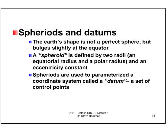
This slide identifies the mathematical representation of the earth's surface. They are spheroid, and datum. These are defined by parameters and are used in mathematical formulae which transform real world ground control coordinates into map coordinates which can be used on hardcopy and in the computer models.
